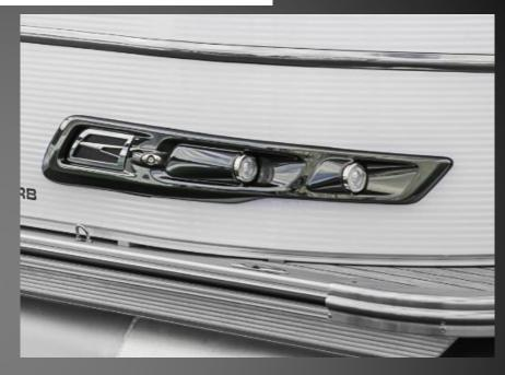
COMPETITOR BOW OR RUB RAIL MOUNT LIGHTS ARE A DAMAGE AND TRIP HAZARD
